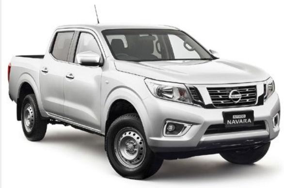
Most efficient ute variant available: Nissan Navara D23 NP300 4x2 Twin Turbo 2.3L 4-cylinder diesel (2015)
