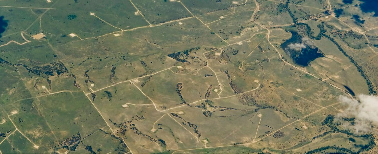
Figure 5: Unconventional gas development requires many individual wells to be drilled over a large area, as seen in this aerial photo of Queensland's Western Downs.
