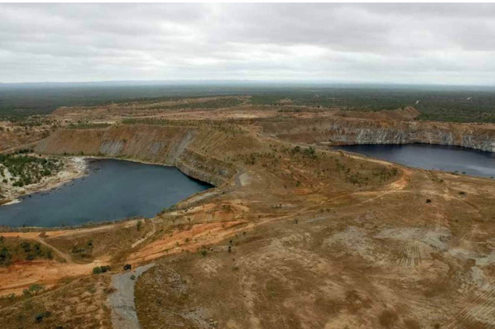
Figure 19: The former Kidston gold mine. Genex Power plans to construct a pumped hydro facility on the site by pumping water from one lake into the next.
