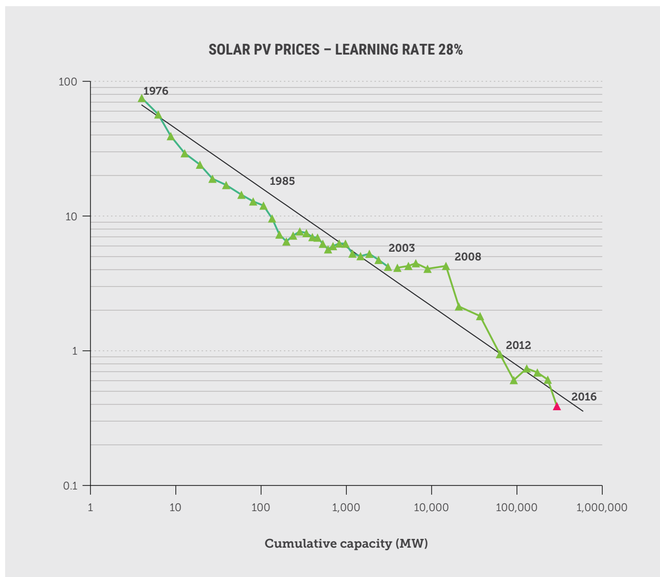
Figure 12: Over the past 30 years, the cost of solar PV has fallen significantly as capacity has increased. Lithium-ion battery prices are falling almost as fast (Figure 13).
