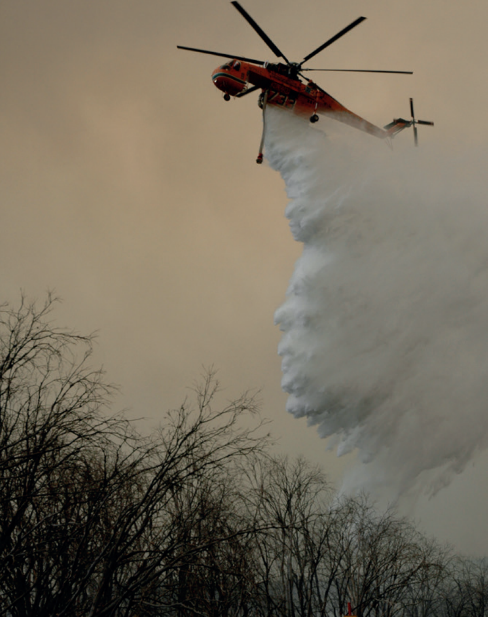
Figure 6: Elvis – the Erickson Air-Crane fire bomber – dumping about 9,000 L of water to assist Australian firefighters. Specialised firefighting aircraft like this are loaned for the bushfire seasons in both the Northern and Southern hemispheres each year.
