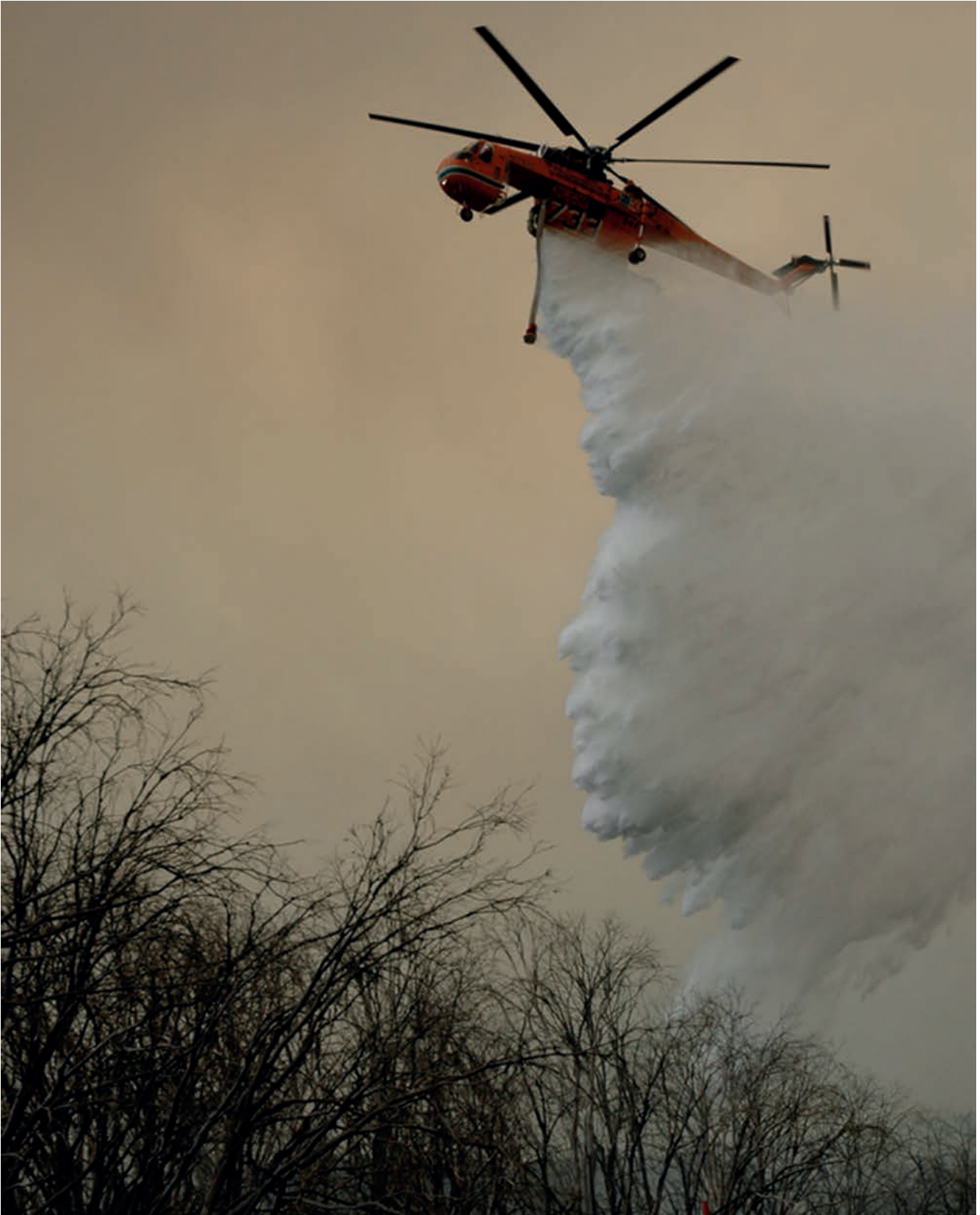
Figure 12: Elvis - the Erickson Air-Crane fire bomber – dumping about 9,000L of water to assist Australian firefighters. Specialised firefighting aircraft such as Air-Cranes are loaned for the bushfire seasons in both the northern and southern hemispheres each year.
